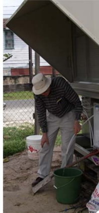
Water-from-air production rate test, Belize City
